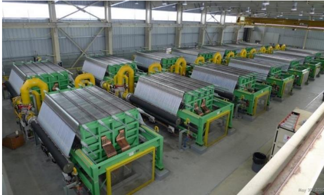
The cell room at the Chemtrade North Vancouver Facility, where chlorine is produced
